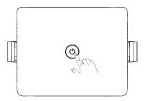
Plug the power cable to the projector. Press power button to turn on the projector.
